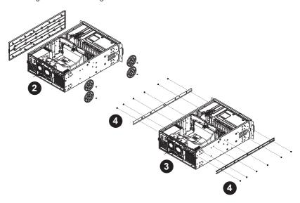
Figure 1: Installing the Inner Chassis Rails
