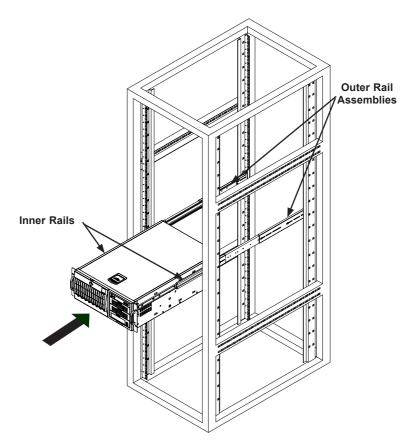
Figure 3: Mounting the Chassis into a Rack
