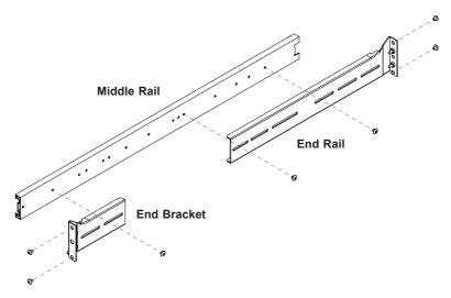
Figure 5-2: Assembling the Outer Chassis Rails
